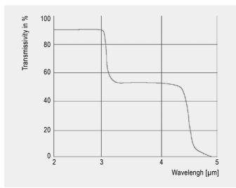
Spectral transmissivity of glass
